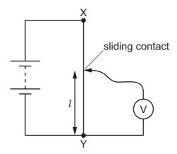
He changes the length of wire *l* by moving the sliding contact along the resistance wire.
